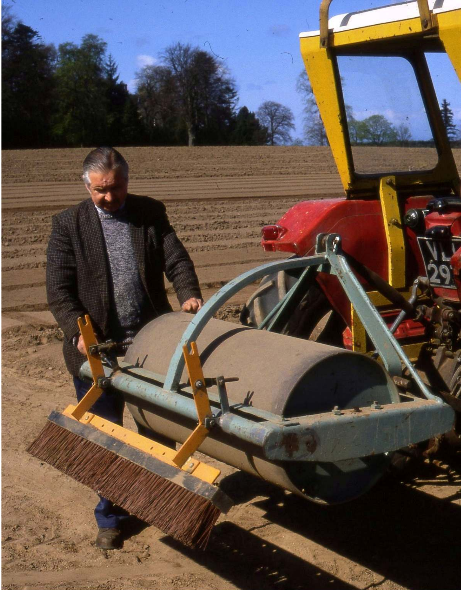
.4 - Rolling and brushing of seedbeds prior to sowing taking place
