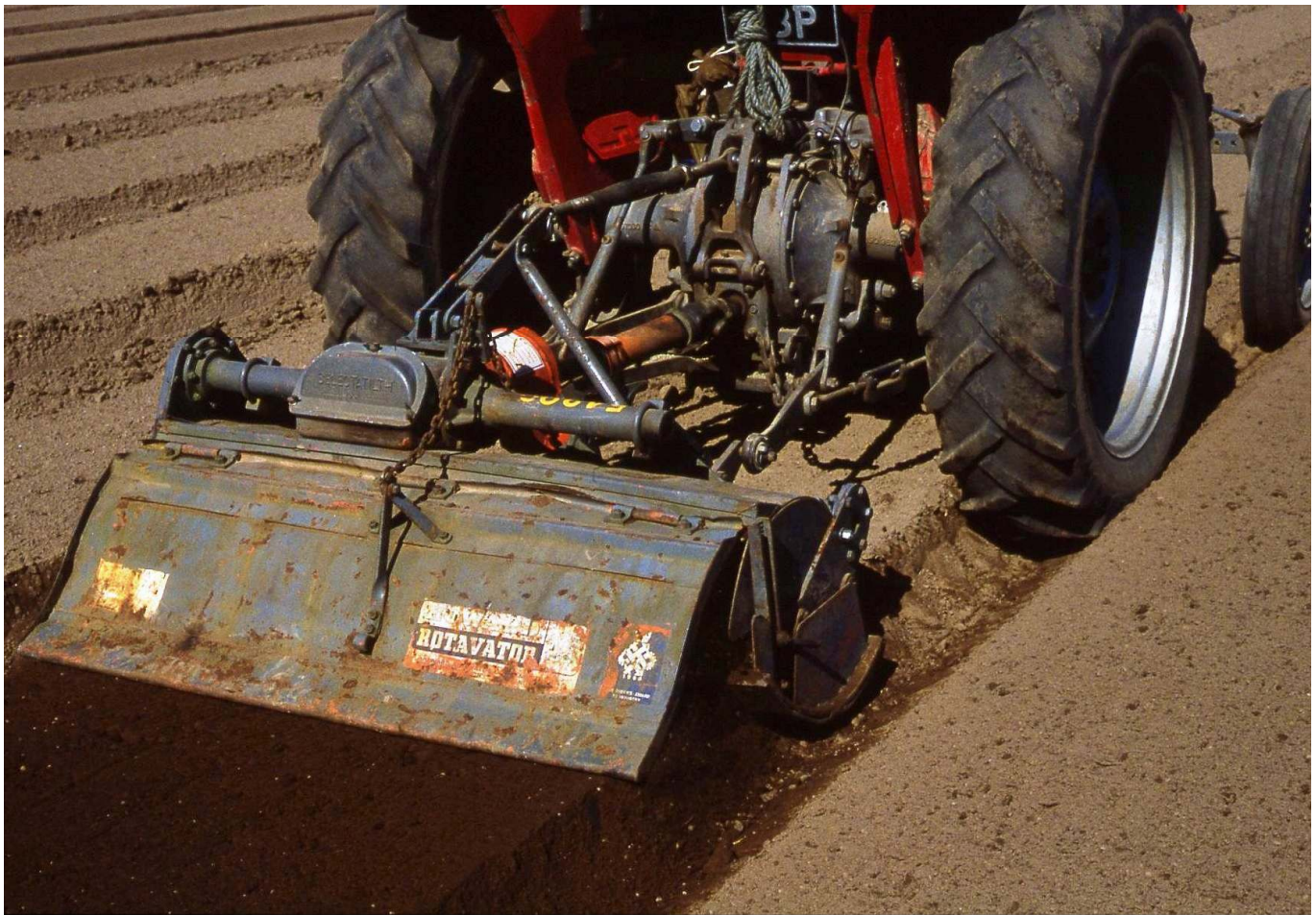
- Rotovating of seedbeds in order to create a fine tilth prior to actual seed sowing.
