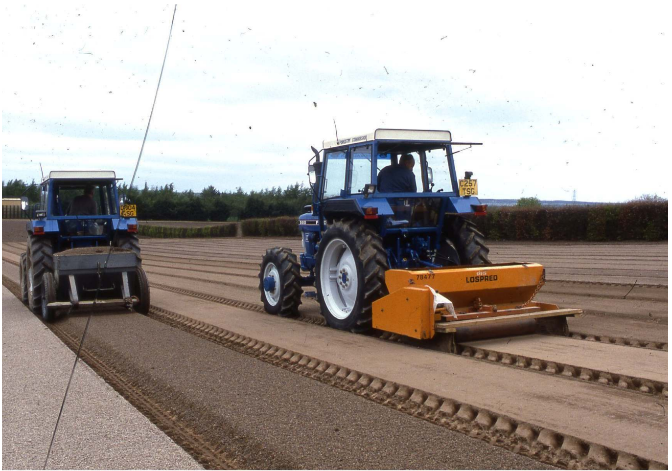
17 - On left applying grit to sown seed bed on right tractor powered seed sower (Sisis seed sower)
