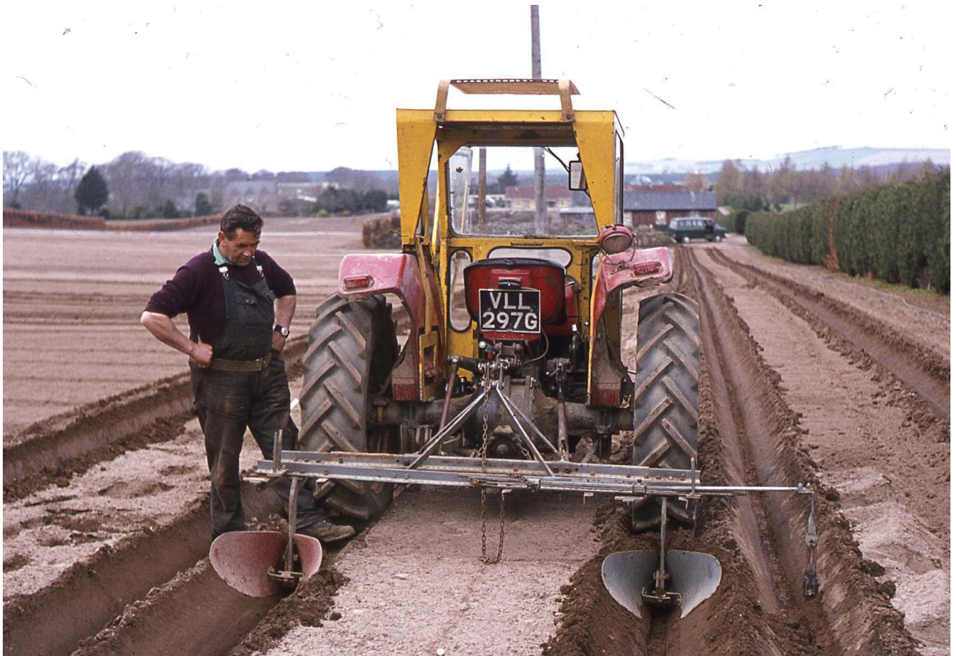
2 - Ridger plough used for forming alleys in order to raise seedbed. Bill McKenzie driver
