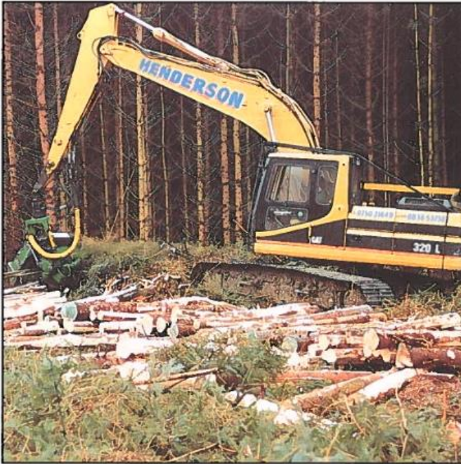
CAT 320L with LAKO 60 Head cutting bars and pulp production 80T/day
