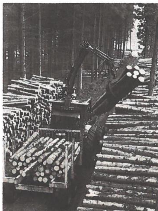
● Contractor's forwarder collects material from the felling site in Laplojd plantation.
