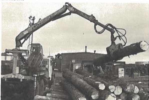
A mobile Highland Bear crane is the specialist sawlog-handling unit. Sawlogs come from as far away as Argyllshire. In mid-April continuing bad weather had meant that, with some forests still inaccessible, stocks were lower than ideal.
