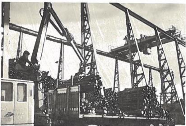
Lorries with self-loaders — here unloading pulpwood — find their loads within an average 70 mile radius. As specialised vehicles they find that they are profitable on this basis, without the need for a revenue-related backhaul.
