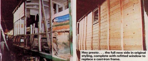
How a "living van" took on a new life . . . in four stages. This is how it looked when Alwyn Rogers first saw it in 1989 . . . but this view hides the real damage (below, left) on the other side, where rotting boards had to be removed.
