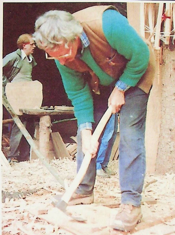
Peter Quelch gets down to it . . . adzing a chair seat, while Eric Rodgers (front) turns chair spindles on a pole lathe.
