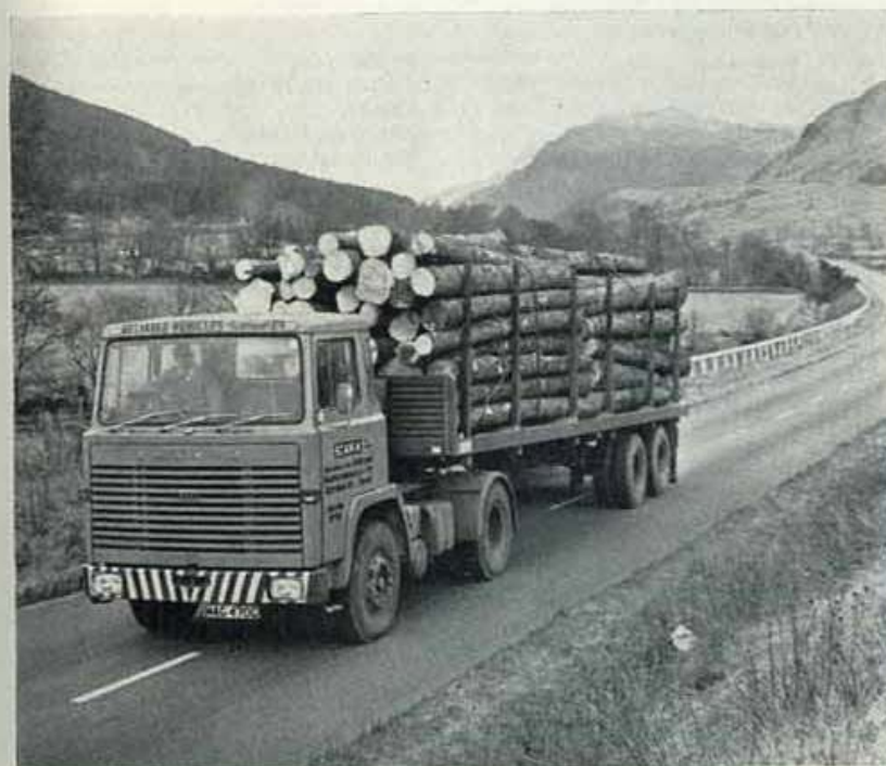
SCANIA LB10 10 ft. Wheel Base Tractor Unit complete with TASKERS 32'6" Long FORMULA 1 Dual Purpose Timber/Platform Semi-Trailer, at 30 tons gross.
