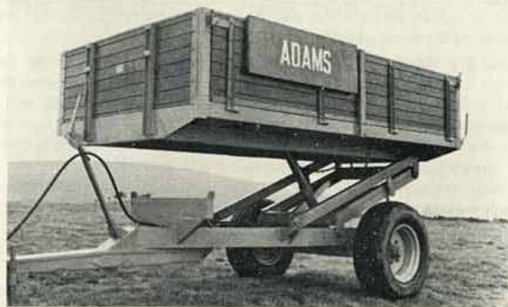
Multi purpose trailer (Tipper) suitable for Stillage. Removable sides, Front and Rear Doors.
