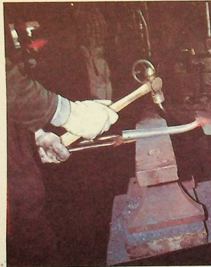
BELOW: Machinery may have taken over from man in the mass production of tools, but when it comes to the final inspection there is nothing to surpass the eye and hand of the skilled craftsman. This spade has been through ten forging stages and is now being tested for shape and balance.
