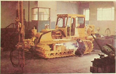
Fitter Brendan Grant uses his welding torch on a Rock Drilling Rig.
