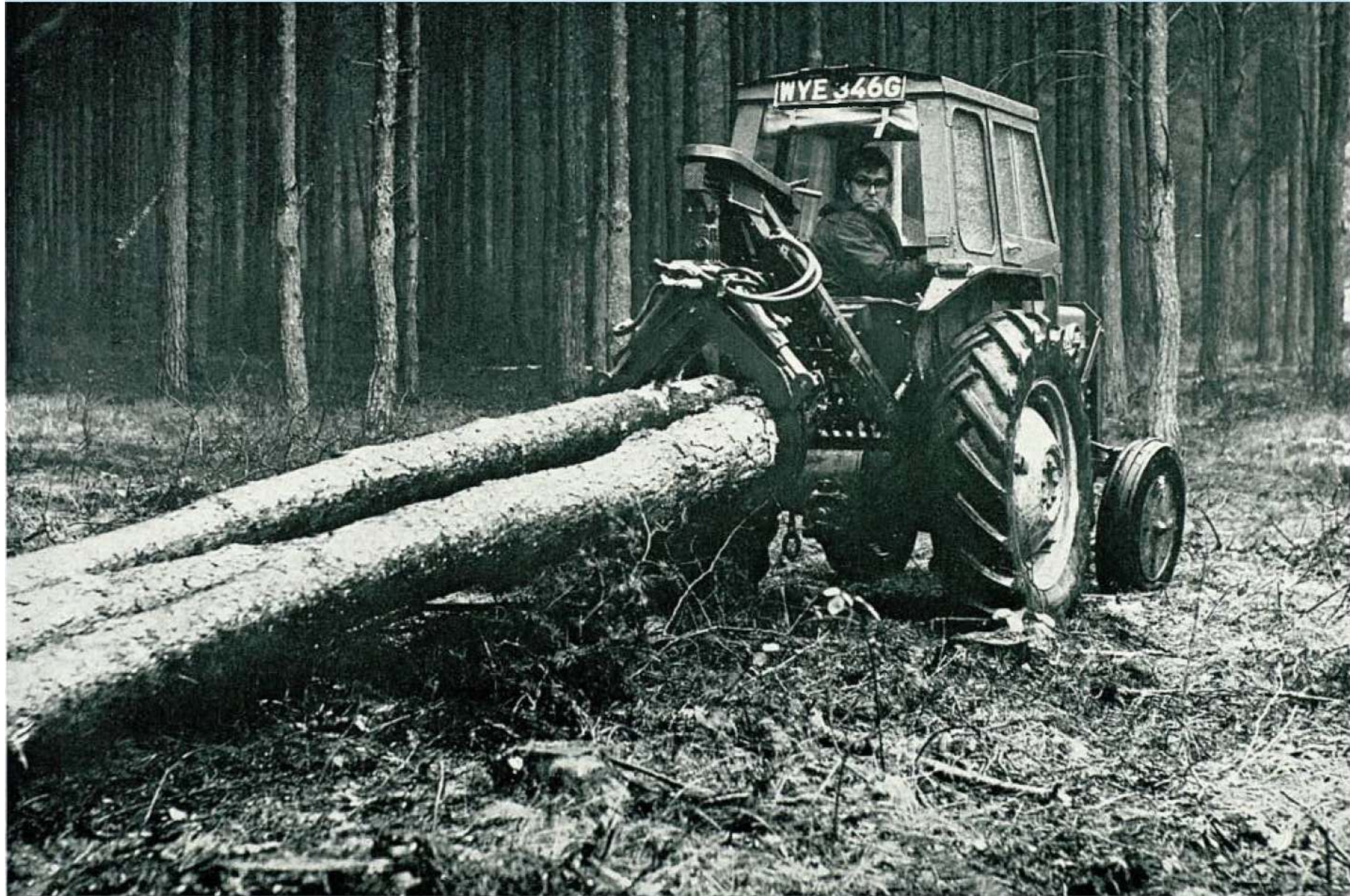
PLATE 5. An agricultural tractor, fitted with hydraulic tongs, hauling pine logs from Thetford Forest in East Anglia. See para 38 UT9209
