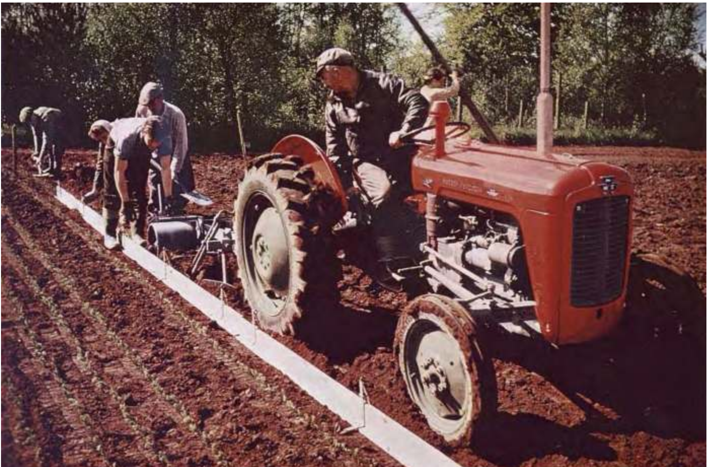
Transplanting seedlings at Ledmore Forest Nursery in Perthshire. The tractor draws a lining-out plough, designed by a Commission forester. This places earth against the roots of trees, held in a trench by boards, and at the same time, cuts the next trench.
