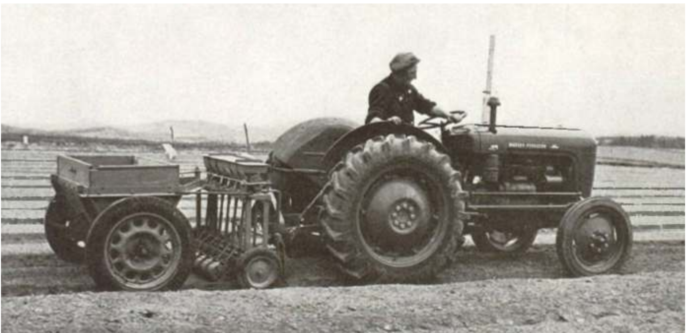
The Ledmore Six Drill Seed Sowing Machine in the 1950s, for sowing seed in drills and covering them
