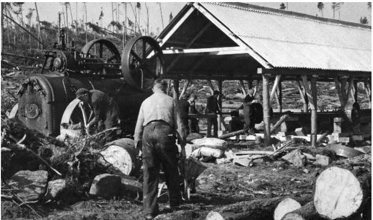
Steam driven mobile sawbench sawing logs from the 1953 windblow on Deeside. This was the last as fixed mills took over. (Sandy Touch)
