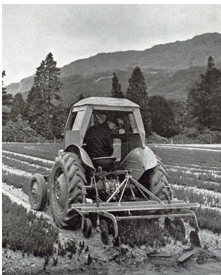
The Ledmore Twin Blade Root Pruner undercutting lodgepole pine seedlings at Glenfinart Nursery.
