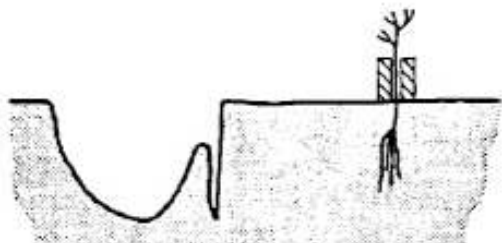
5. New vertical face cut by rear disc.
