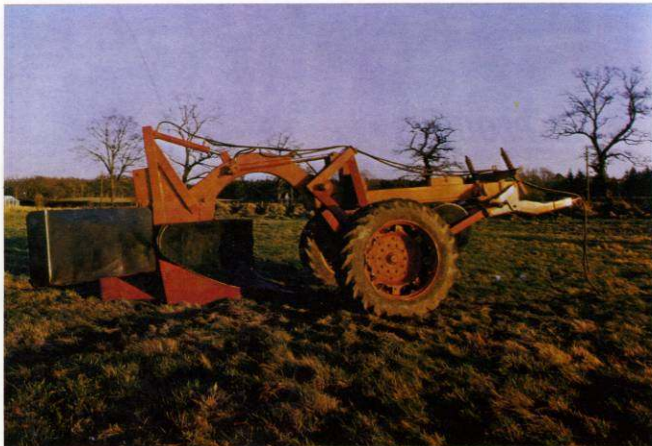
Parkgate Trailed Deep Tine & Draining Plough Arched Beam Model, shown with a single throw draining mouldboard.
