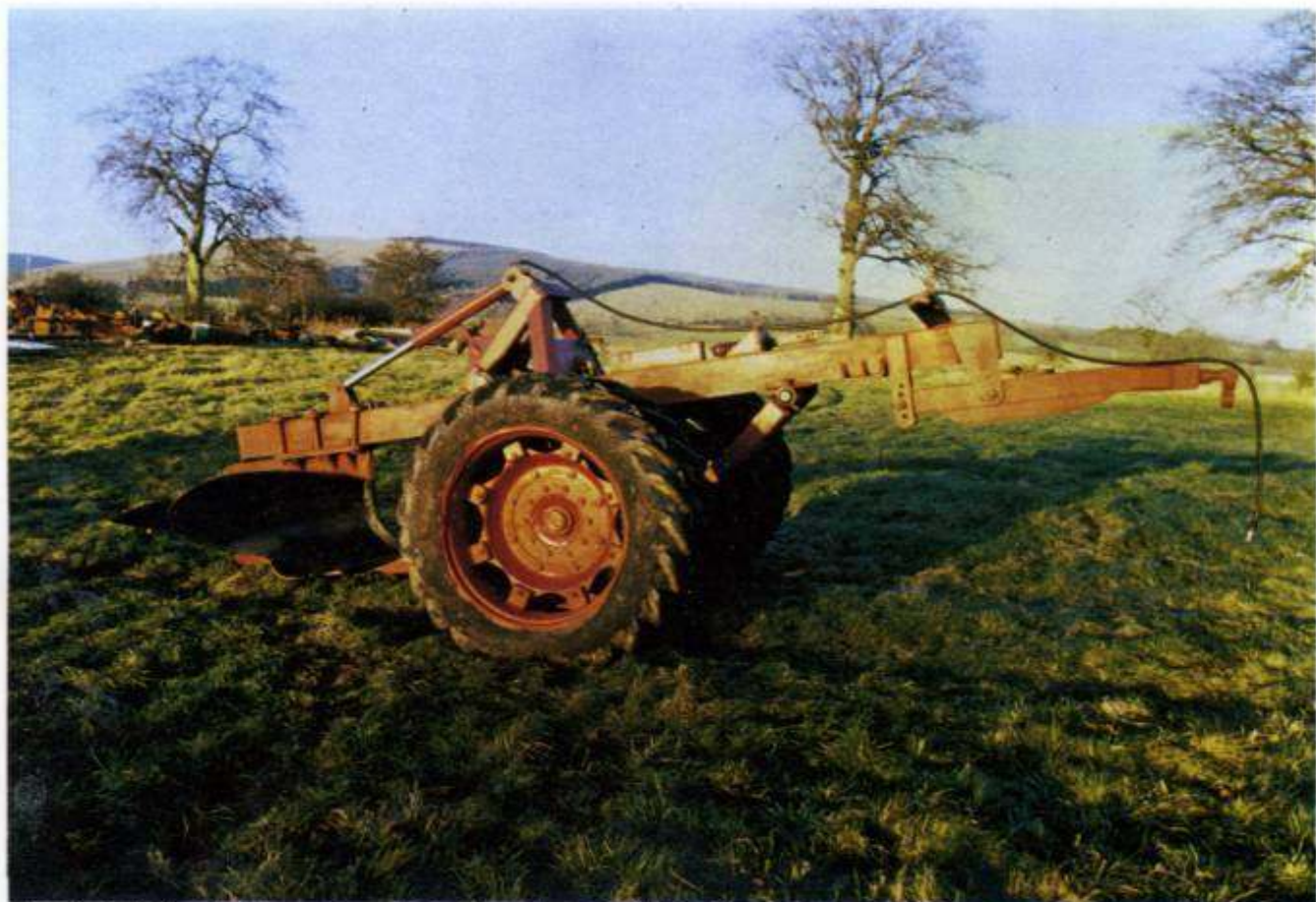
The Trailed Plough fitted with a single throw tine mouldboard
