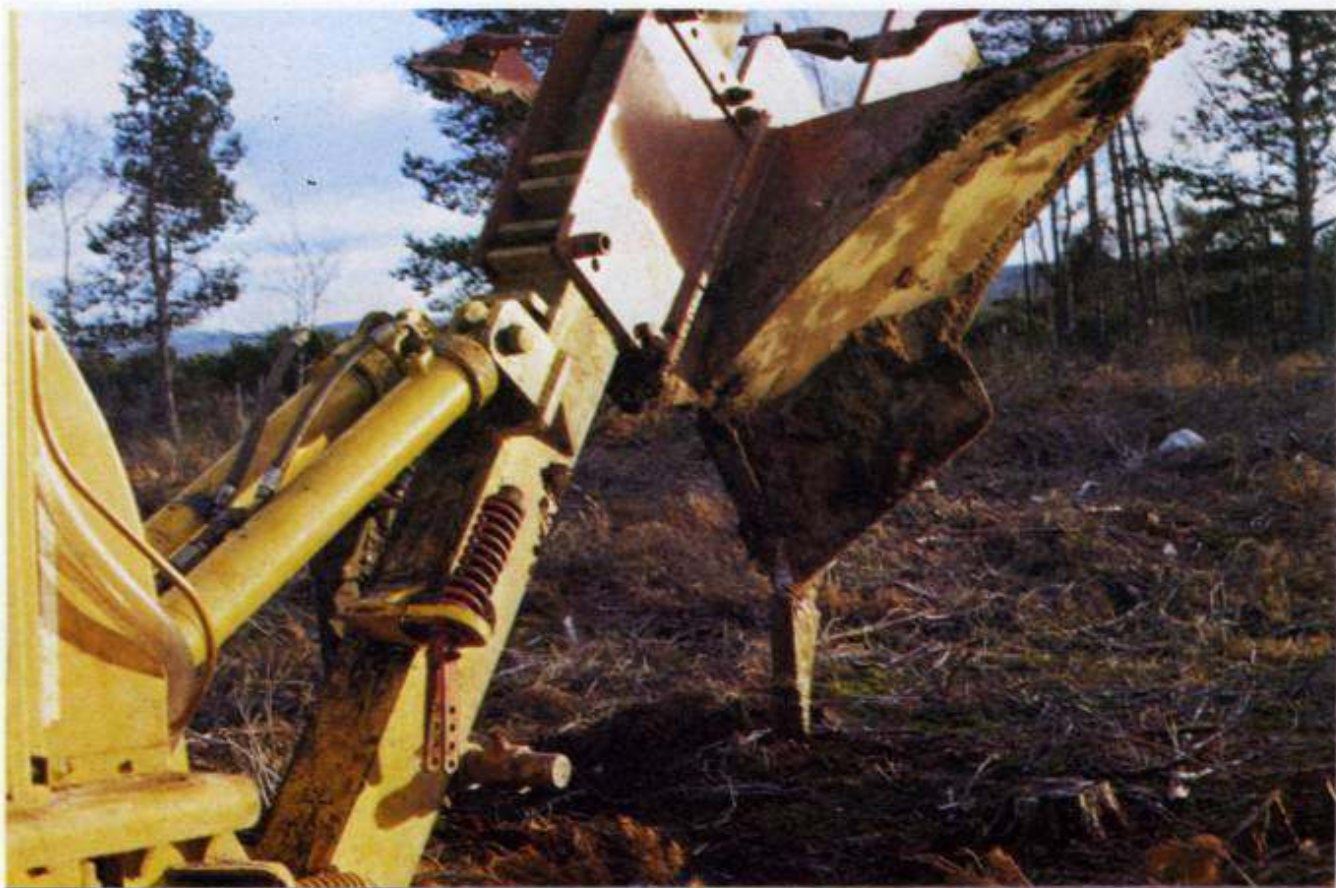
The Mounted Plough fitted with a Double Throw (Deep) Tine Mouldboard.
