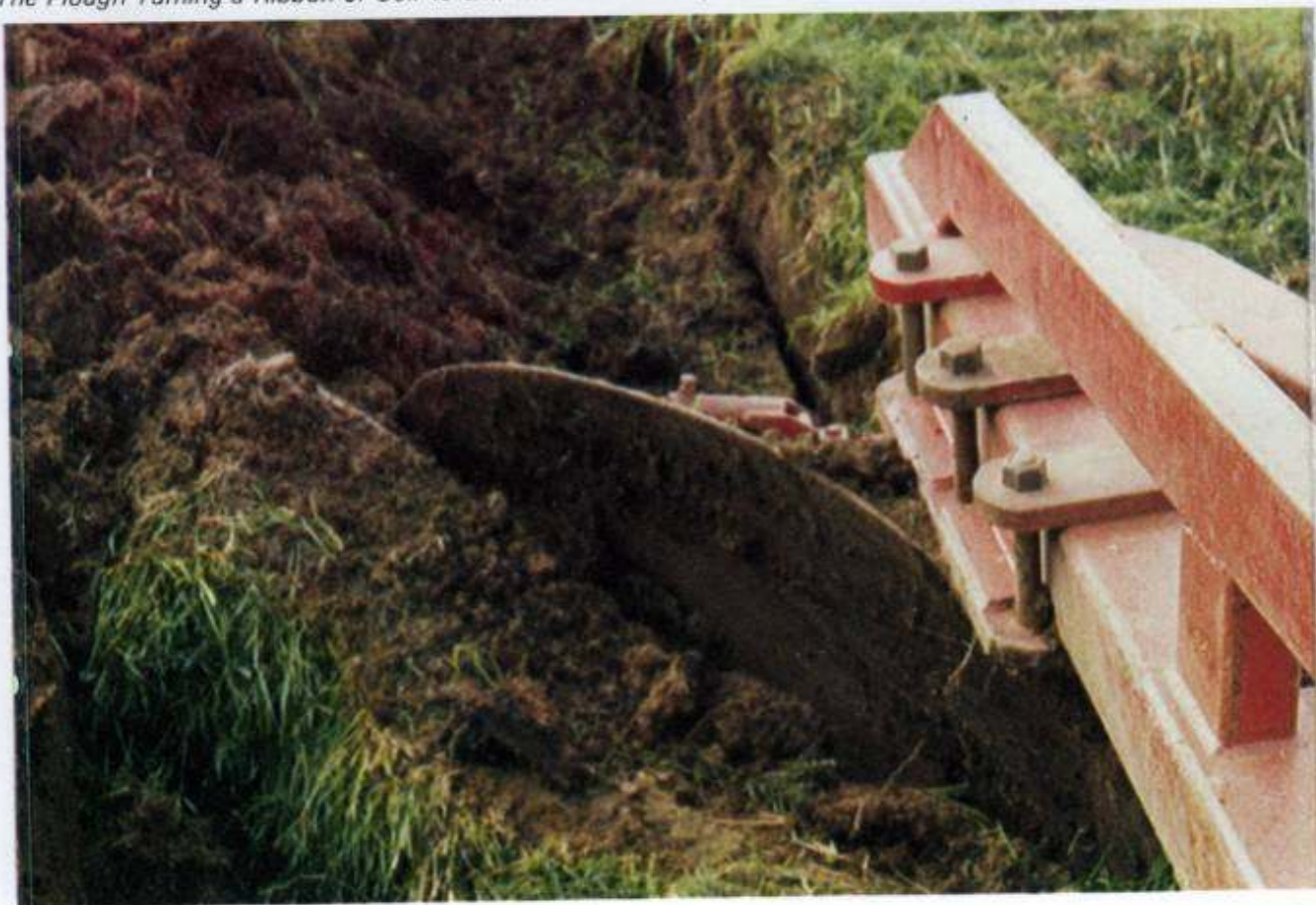
The Plough Turning a Ribbon of Soil 40 cm. wide 30 cm. deep.
