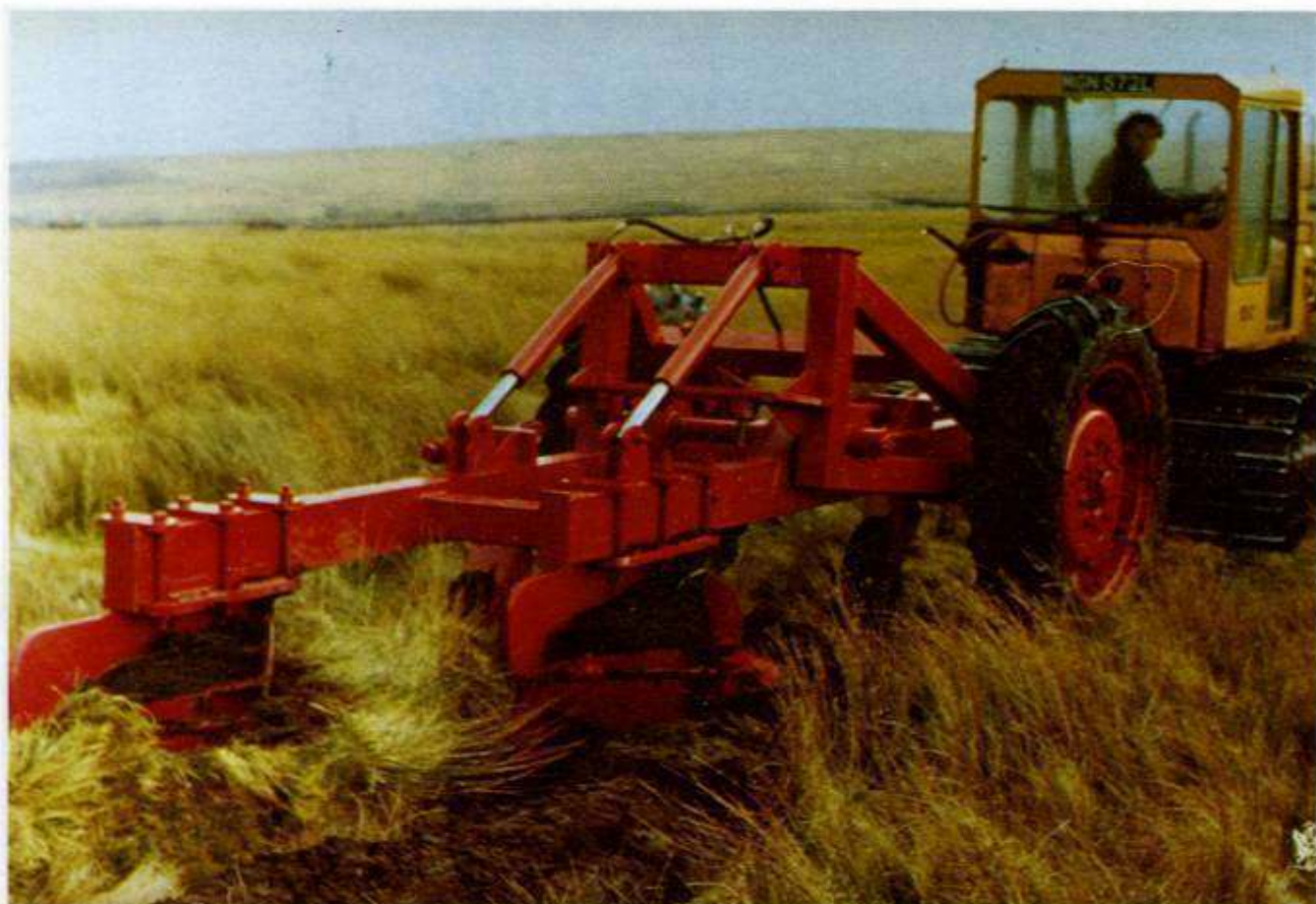
Twin Furrow Trailed Plough in operation giving complete cultivation down to depths of 45 cm.
