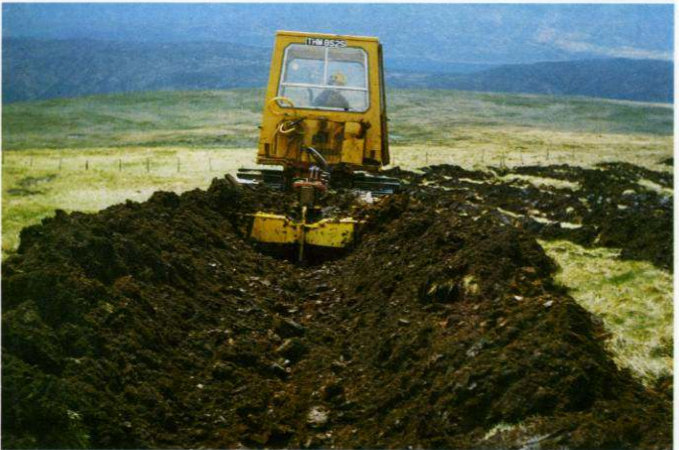
The Mounted Plough in use with a Double Throw Tine Mouldboard
