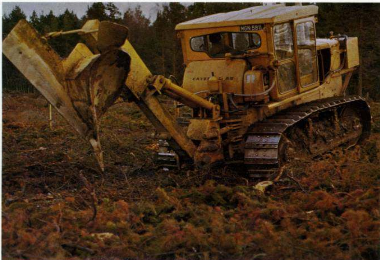
The Mounted Plough in the raised position fitted with a Single Throw (Deep) Tine Mouldboard
