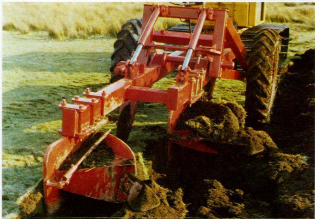
Twin Furrow Trailed Plough in operation giving complete cultivation down to depths of 45 cm.
