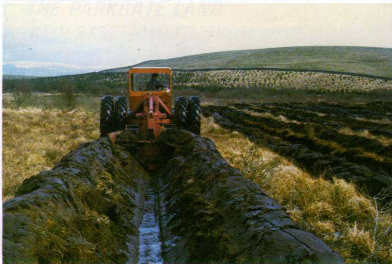
The Trailed Plough with a Double Throw Turfing Mouldboard.
