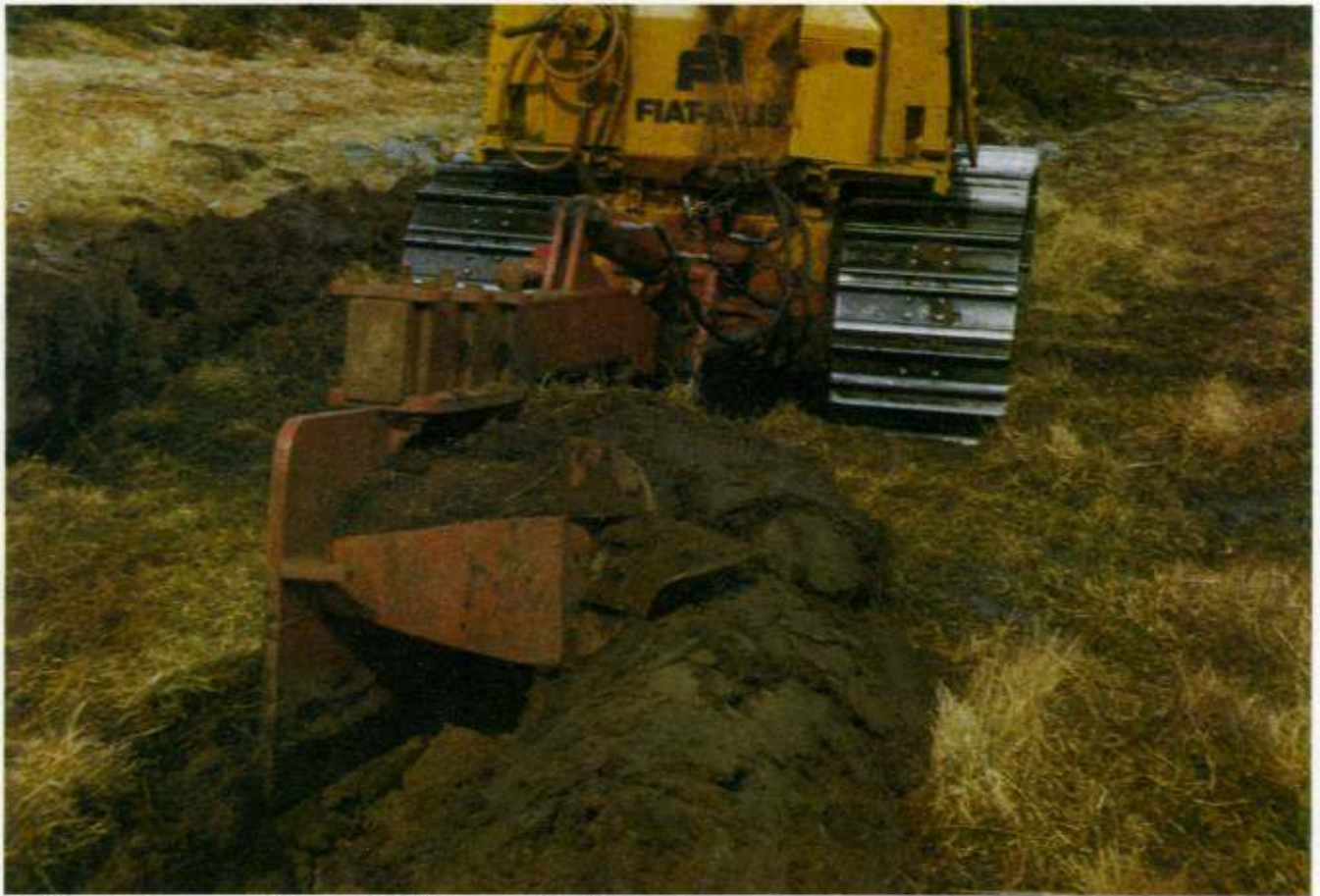
The Plough Turning a Ribbon of Soil 45 cm. wide, 45 cm. deep
