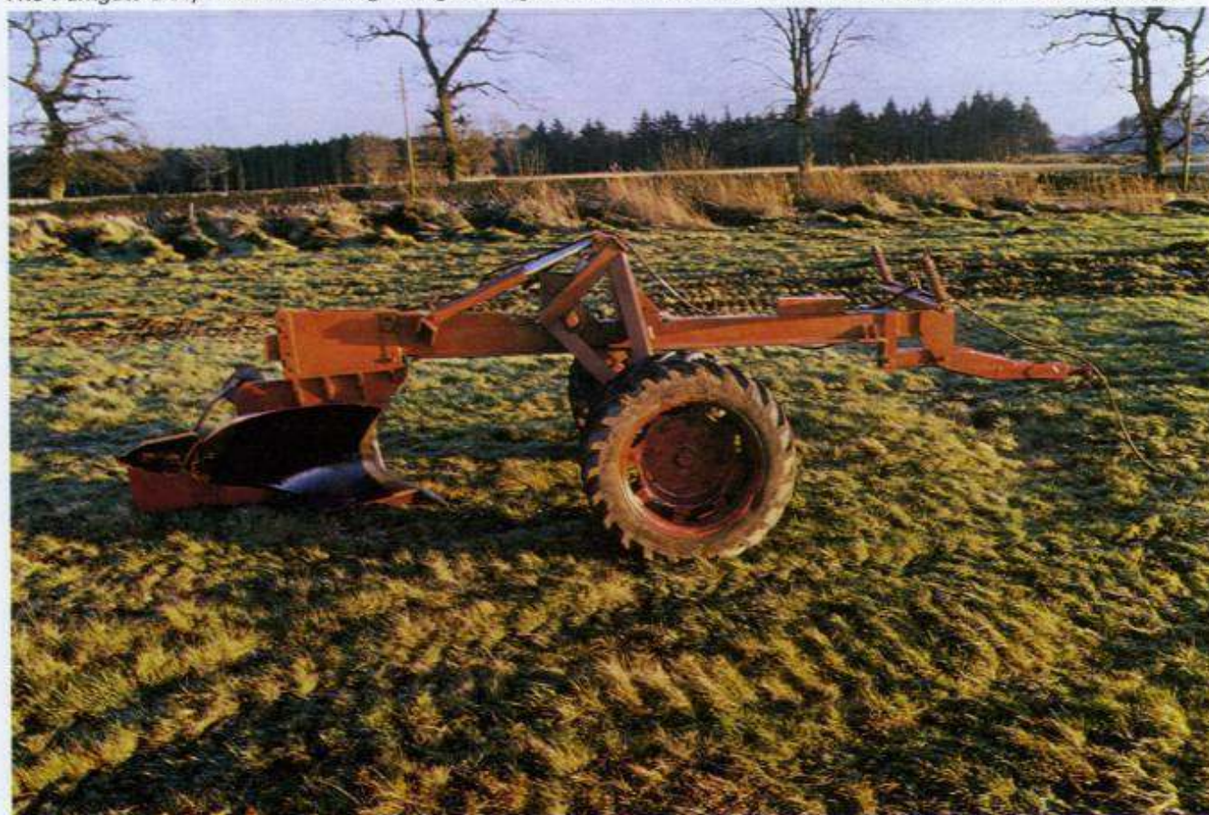
The Parkgate Deep Tine & Draining Plough Straight Beam Model, shown with a double throw tine mouldboard.
