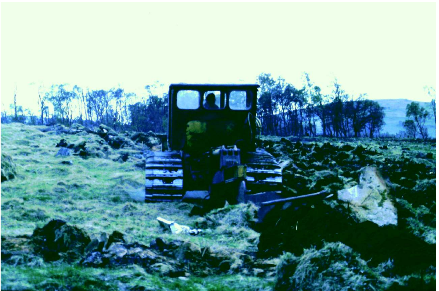
These two photographs show a Sickle Plough mounted on a D7 Crawler Tractor. This was a heavy duty Single Throw Plough, which was used to plough areas of ground that had been cleared of standing Birch in the Culltullich area below Burnside. This was the most powerful ploughing rig you could get at the time and was used on clearfelled sites.
