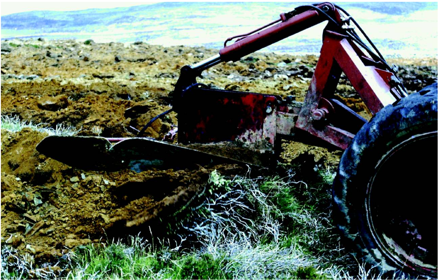
This photograph demonstrated the action of a double mould board plough with this particular plough mould board being developed by Andrew Allan, throwing out a plough furrow like the bow wave of a ship, with the furrow “rolling over” with no straight edge cut formed and a smooth slope down to the base of the furrow, as can be seen in the photograph below. The hydraulic ram allowed the mould board to be held level at a set height.
