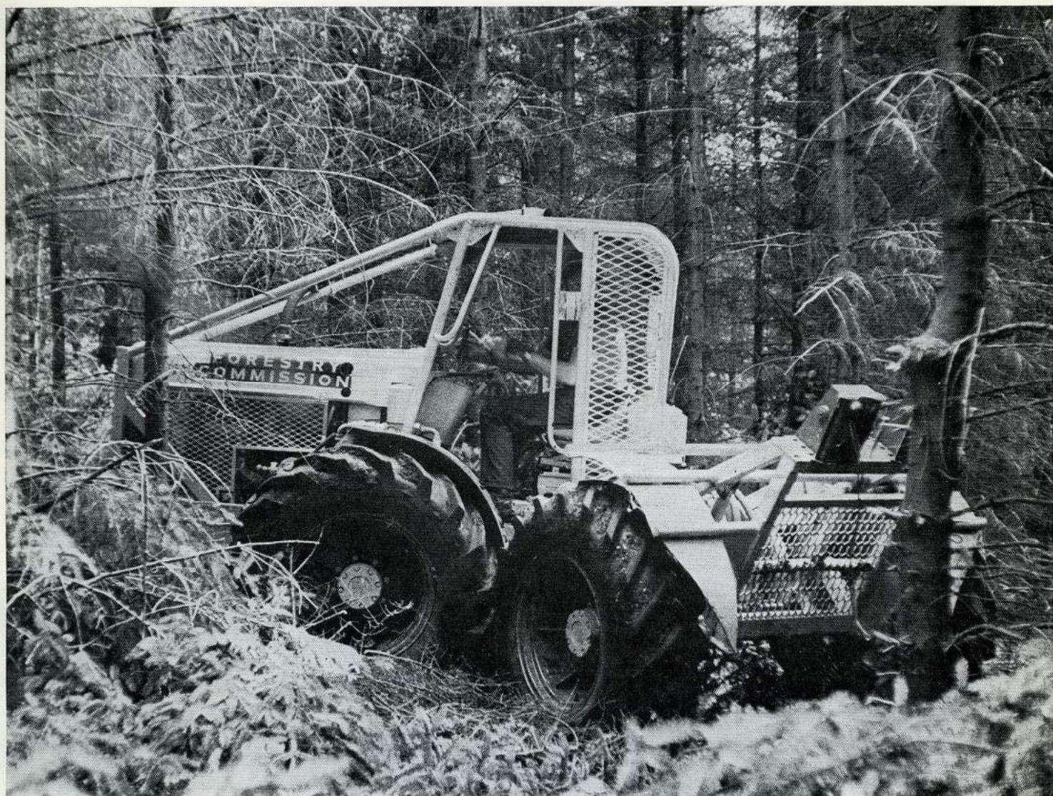
Plate 6. The Mark III on trial in thinning Sitka spruce at Greskine Forest, Dumfries-shire. Note the "tiller" steering.
