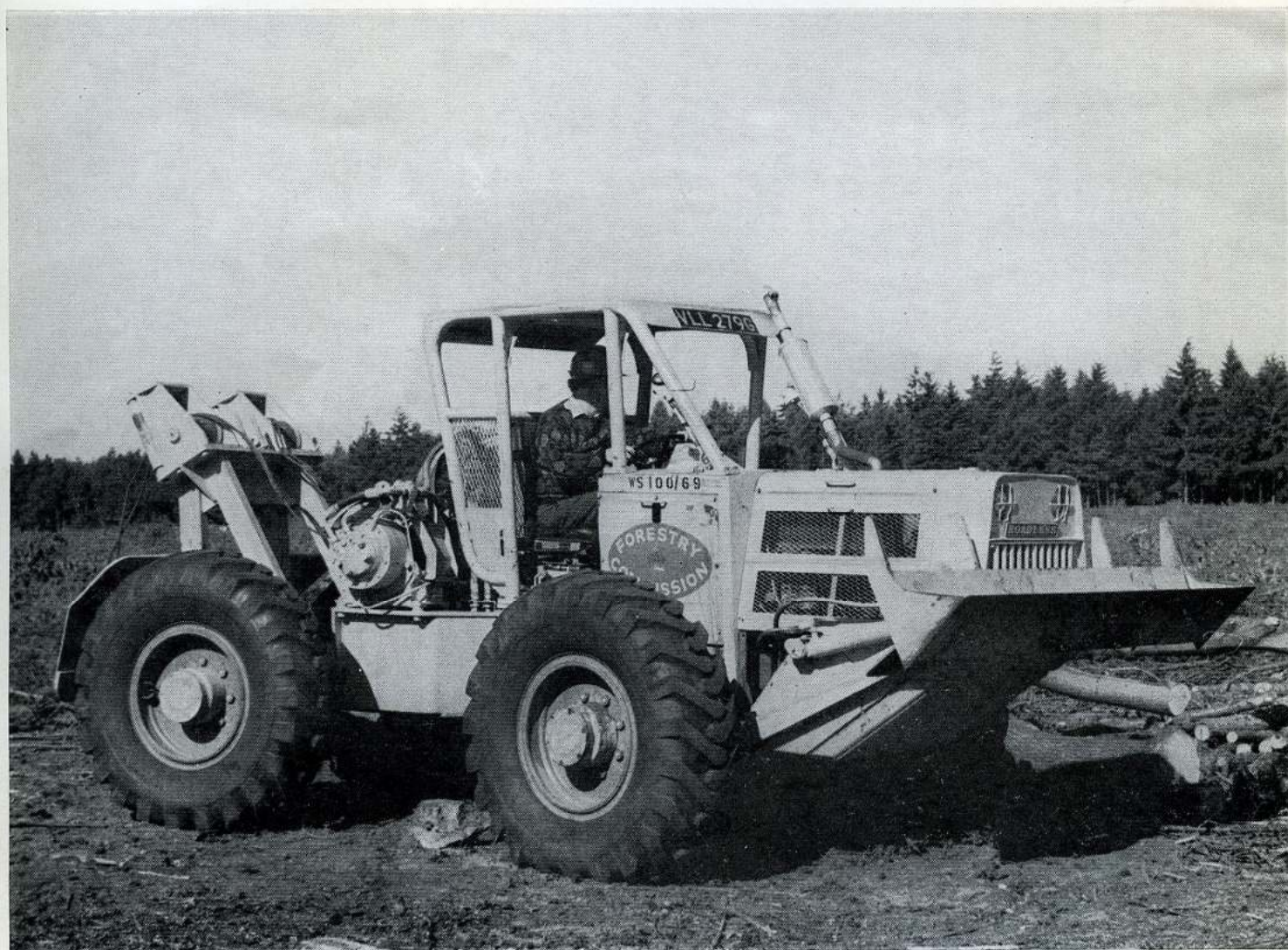
Plate 2. The very first (75 brake-horse-power) hydrostatic forest tractor.
