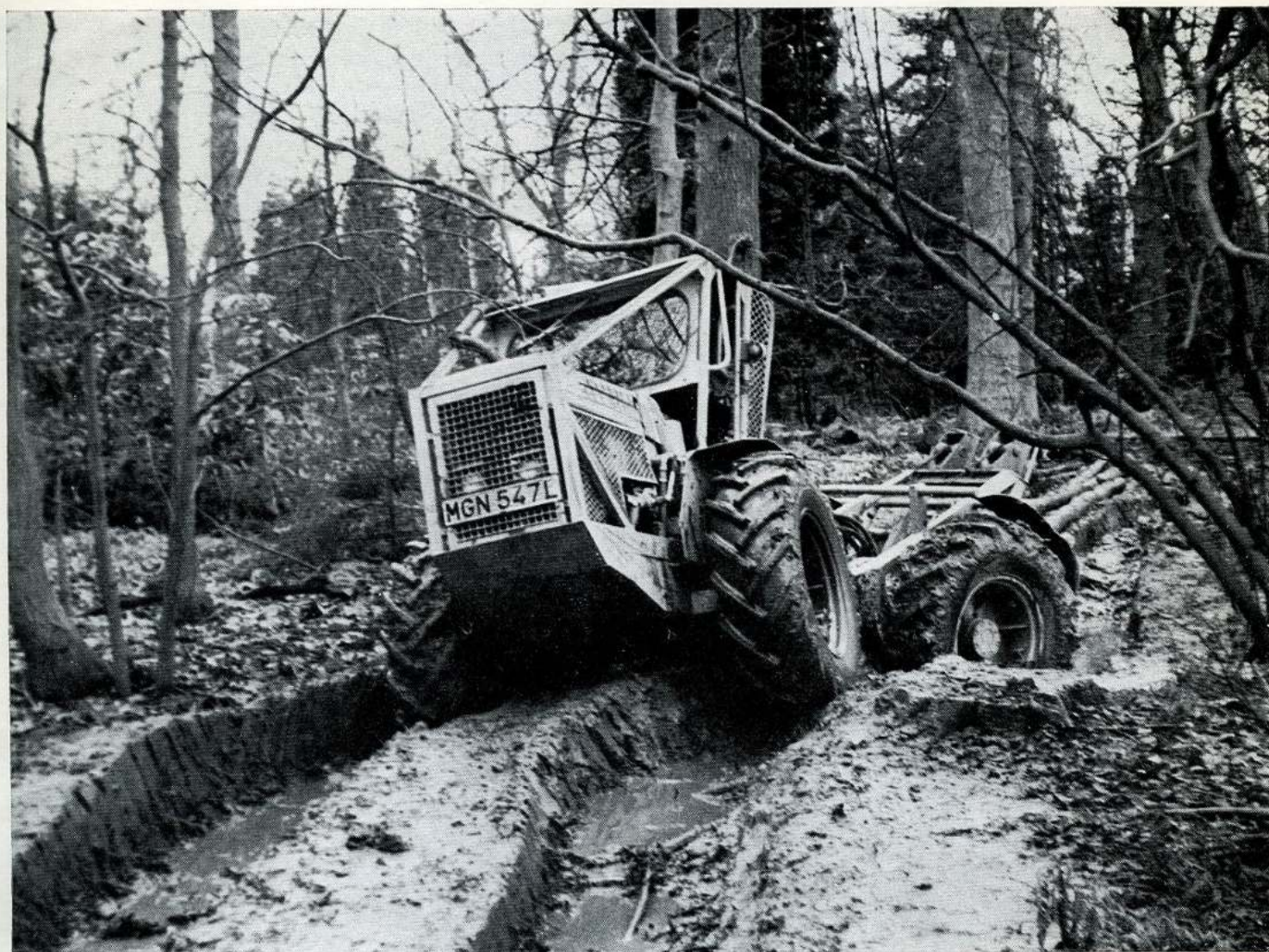
Plate 4. An indication of the high ground clearance and the advantages of the articulated chassis can be gleaned from this photograph of the Mark III.
