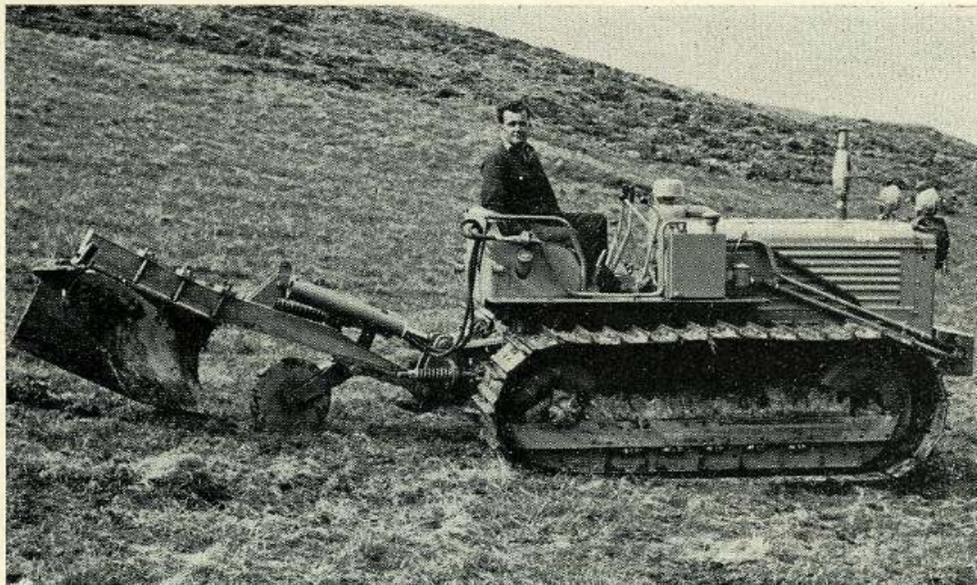
Pl. 3 Prototype plough with hydraulic lift. To avoid overloading in the rear end of tractor by fitting a winch, a hydraulic ram is used to operate the plough. Greskine Forest. (Forestry Commission A2826).
