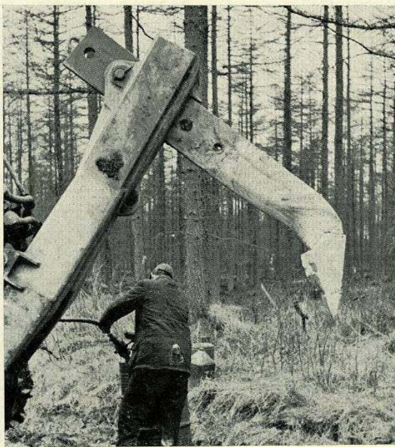
Pl. 5 The Danish Tolne plough. One of the original ploughs for which all but a seat for the operator have been reassembled. Thetford Forest 1975. (Forestry Commission).
