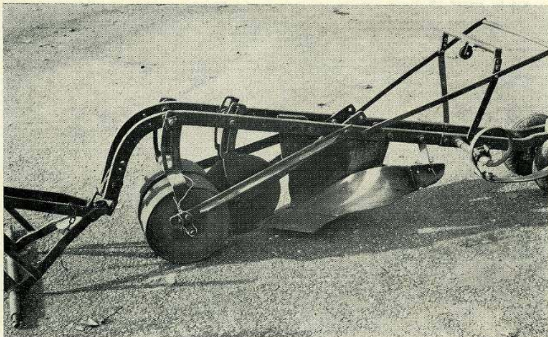
Pl. 5 The Danish Tolne plough. One of the original ploughs for which all but a seat for the operator have been reassembled. Thetford Forest 1975. (Forestry Commission).
