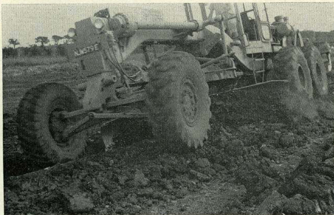
Pl. 10 A large motor grader creating Riggs and Furrs by successive sweeps. First trial on the site of the present M6 in Cumbria 1970. (Forestry Commission).
