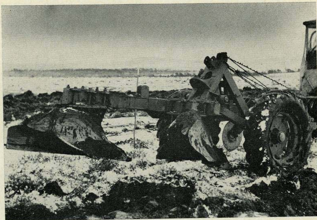
Pl. 18. The earliest twin furrow plough used for ploughing fire traces in South Scotland. (Forestry Commission).
