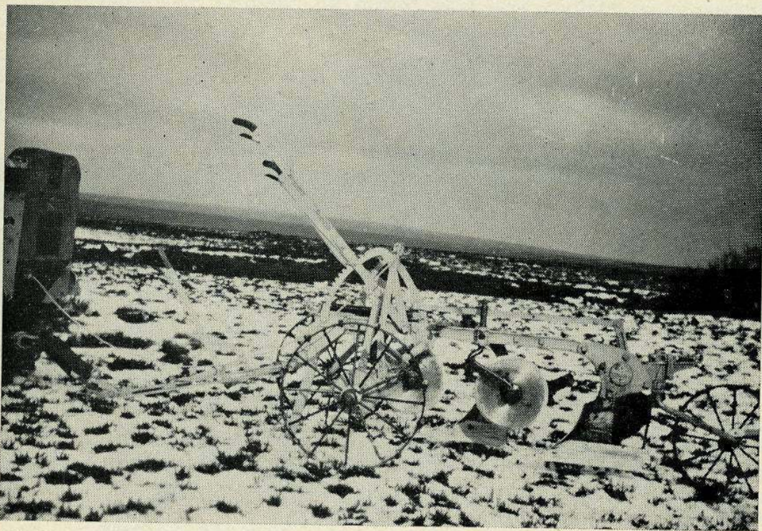
Pl. 6. Ransom two-furrow plough (Two-trac) which incorporated discs. (F.C. F266).
