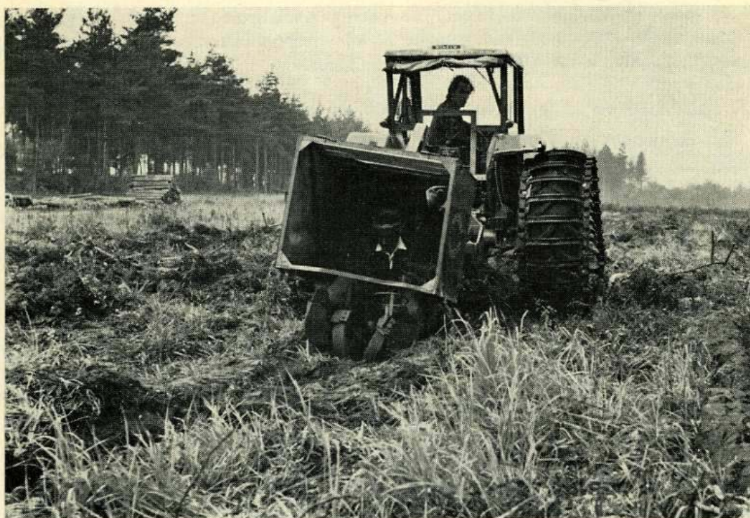
Pl. 6 The Finn planter which was tried but failed to work on ploughing. (Photograph: Forestry Commission).
