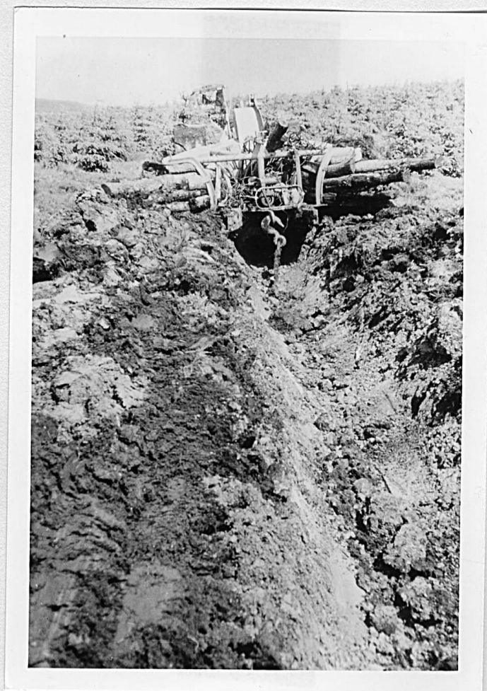
PLATE 5. PLOUGH FROM REAR. NOTE OAK EXTENSIONS. SMALL WINCH MOUNTED ESPECIALLY FOR DEBOGGING SITUATIONS TO HAUL MAIN ROPE. DRAIN IN PEAT OVER CLAY
