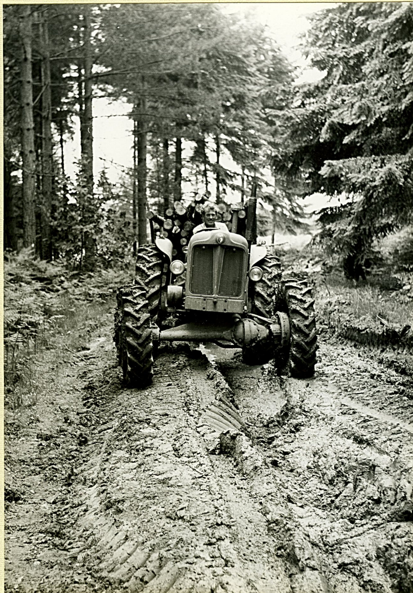
THE MANUAL ROADLESS 4 WHEEL DRIVE CONVERSION ON A FORDSON HAULING TIMBER ON A TRAILER OVER A WET CLAY RIDE AT ALICE HOLT
