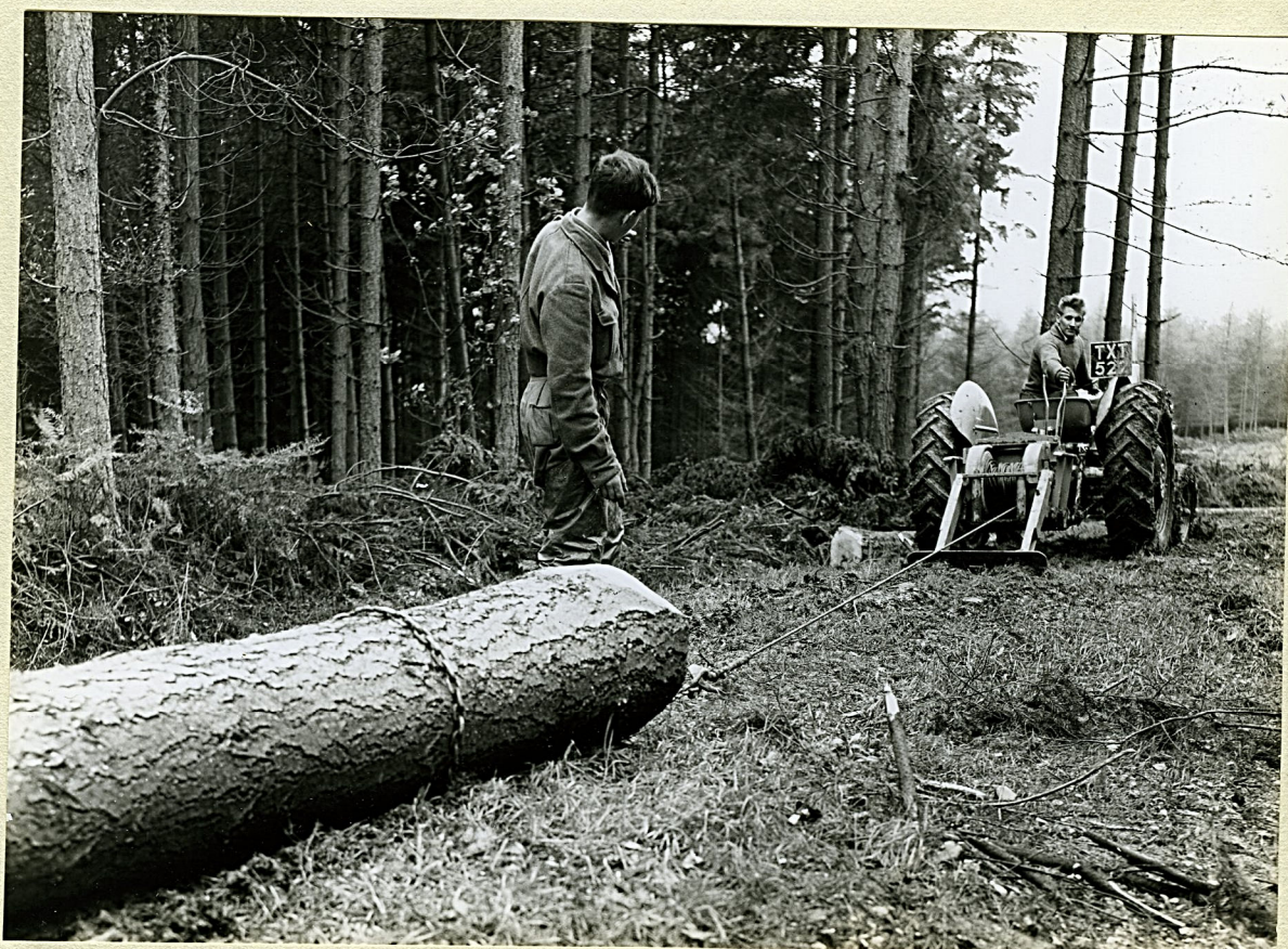
Photograph 2. The winch on the 3 point linkage of a Ferguson 35 tractor hauling timber at Alice Holt.
