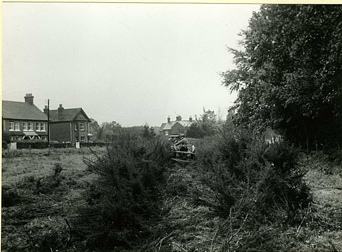
Photograph 2. Showing the passage made through a dense patch of gorse by one passage of the Wolseley Swipe.
