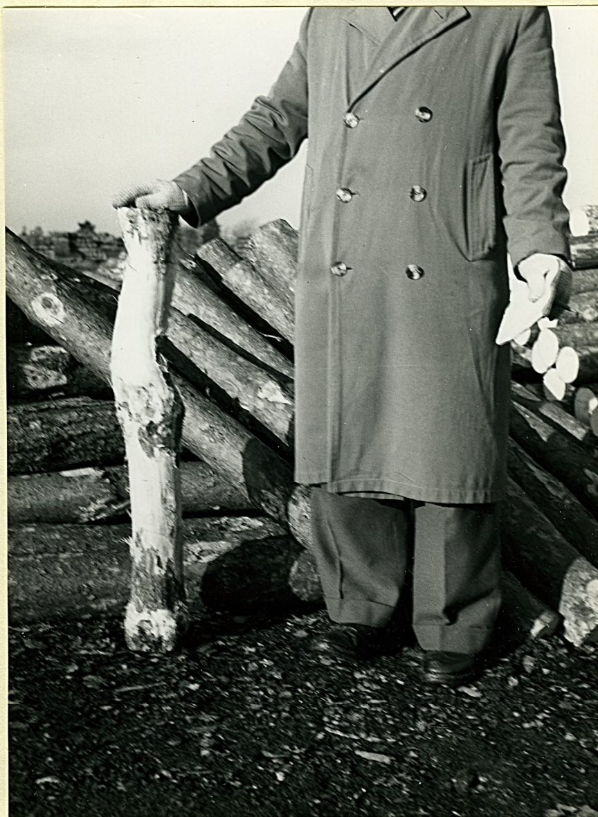
2. A crooked prop after passing through the machine. It was reasonably well peeled but a few patches of bark will be seen to have been left behind.
