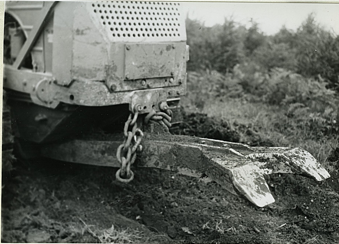
Photograph 1. The S.B. Stumper shown mounted on the front of a German Hanomag tractor. In this photograph the cable from the winch for raising and lowering the tool, is concealed by the chains which, in the operating position, limit the traverse of the tool.
