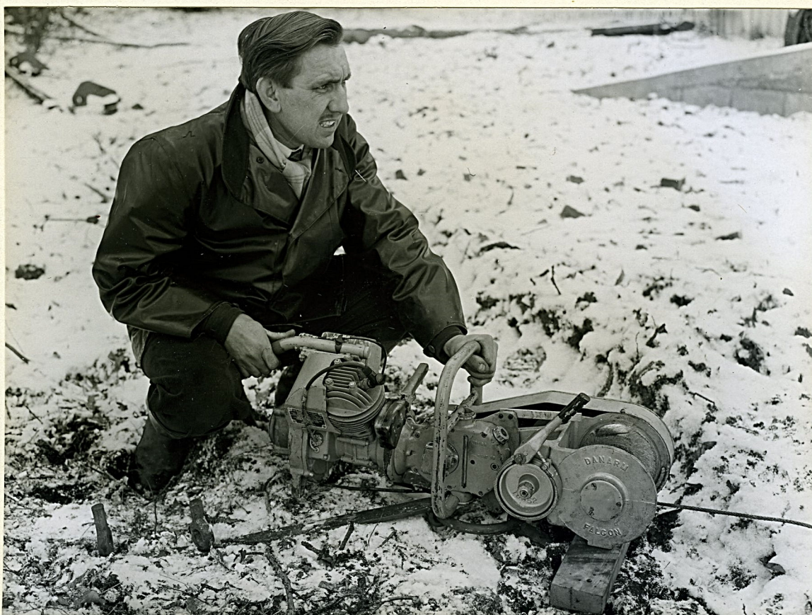
The Danarm Falcon winch in action. Note the ground anchor which forms a V on the ground. One leg of the anchor can be seen with two pins in use. The operator is able to control the winding of the cable on the drum by using the rear handle as a lever.
