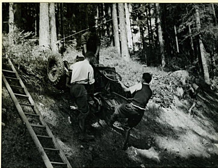
5. The Kupfer winch winching itself up a steep slope.
