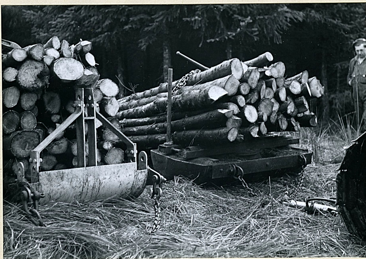
2. The two sledges seen together (the tub sledge on the right) ready for dynamometer tests on grass.
