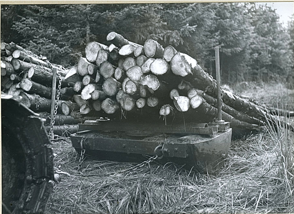
1. The tub sledge with a load of 1 Ton. The hauling chains can just be seen attached to the front face of the sledge.
