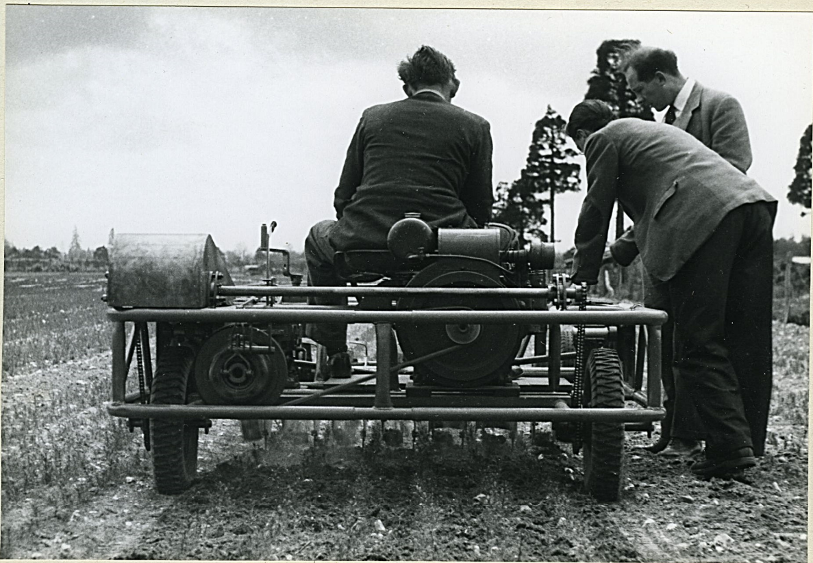
Photograph 2. Rear view of the machine in operation. The revolving blades can be seen below the machine with the rows of plants passing safely between them.
