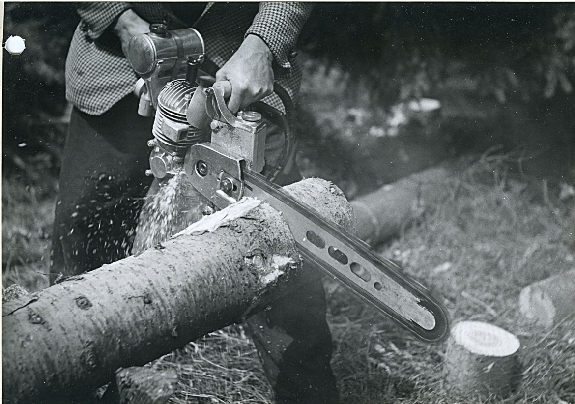
PHOTOGRAPH 1. - Cross cutting with the JO-BU junior saw.
