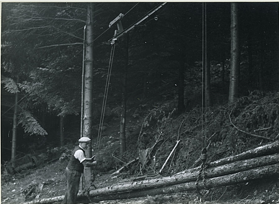
PHOTOGRAPH 1. Showing the lifting hooks pulled down and attached to the load ready for lifting.
