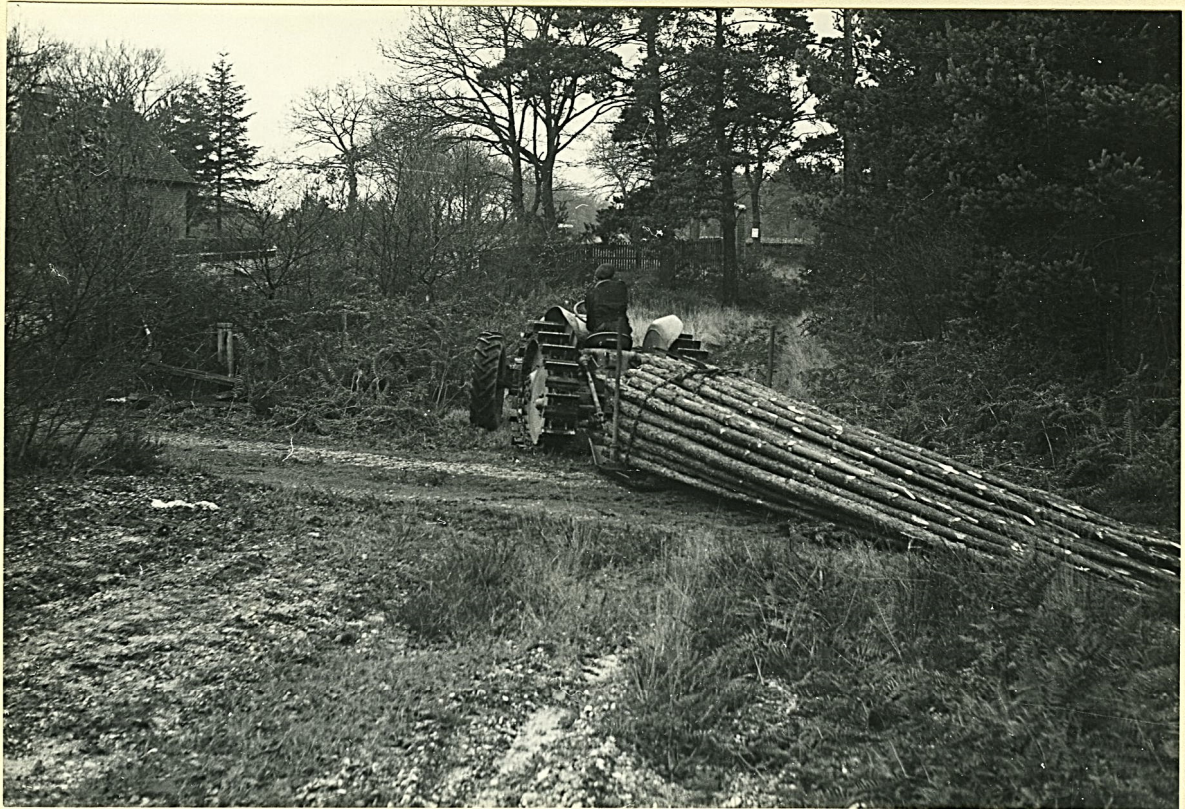
PHOTOGRAPH 2. Showing the sledge carrying a 2 ton load on a forest ride.
