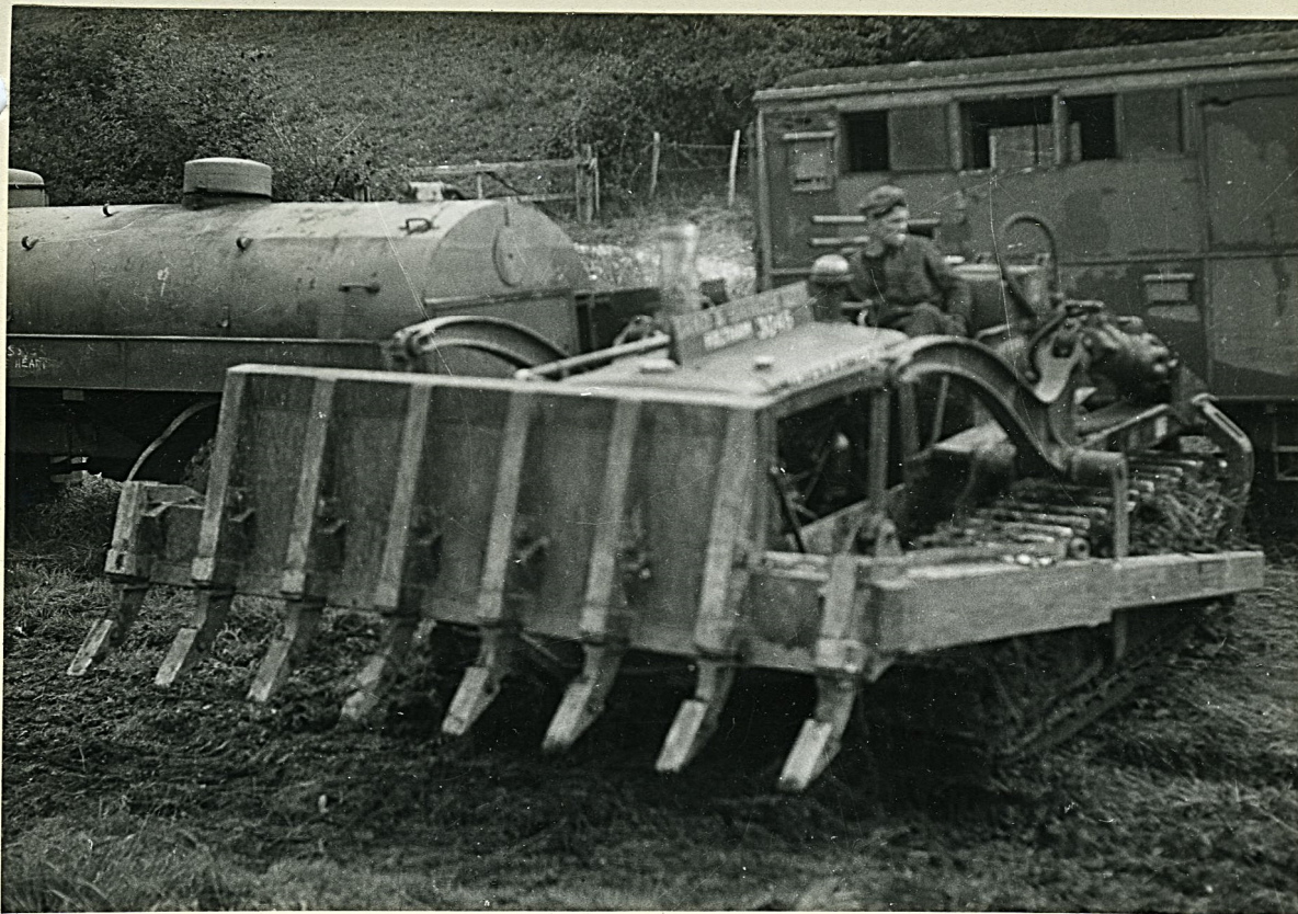
PHOTOGRAPH 1. The grubber blade mounted on a tracked tractor T.D. 14.
