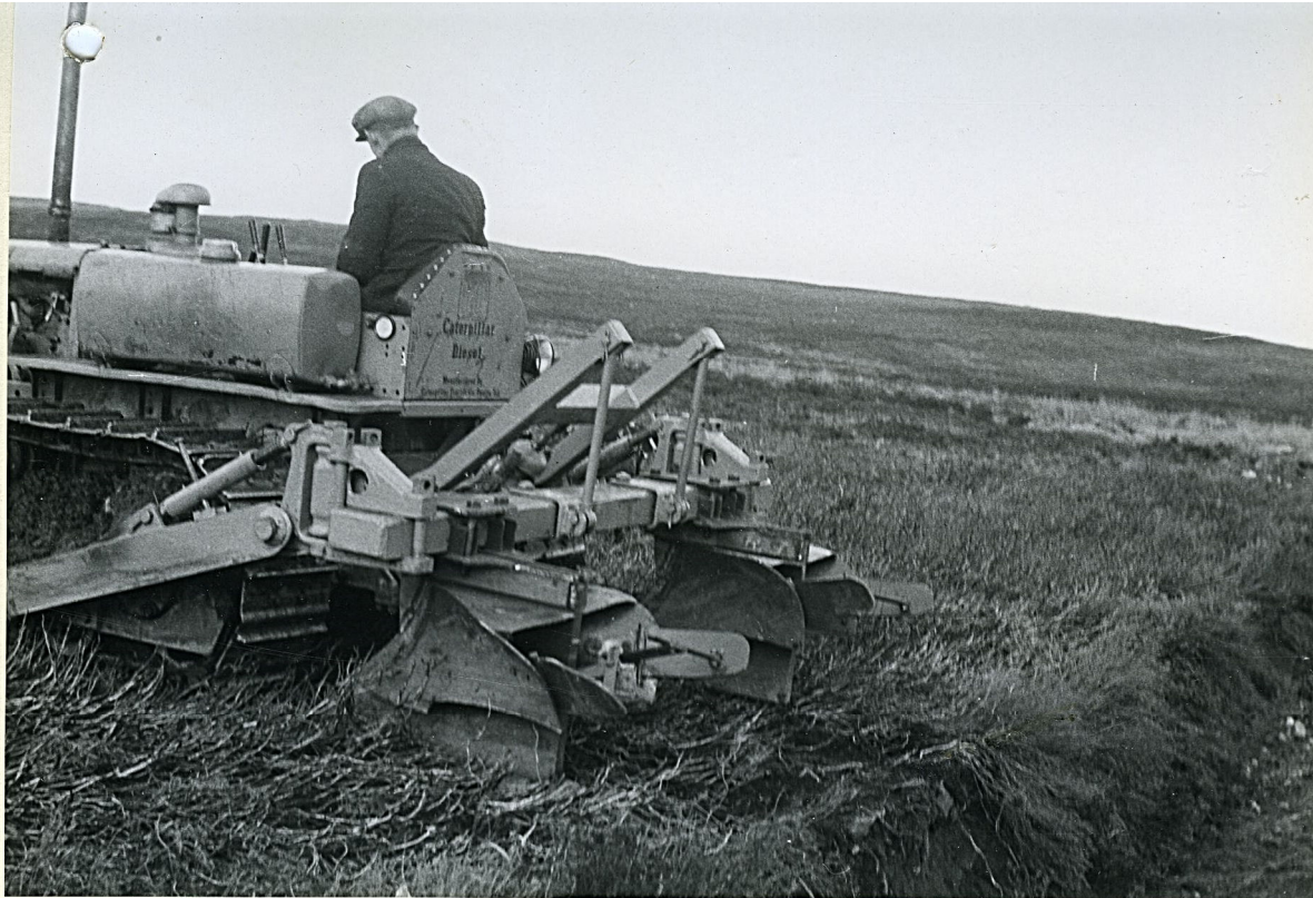
PHOTOGRAPH 1. A D4 tractor with mounted toolbar fitted with two double throw ploughs for ploughing at 5 ft. spacing.
