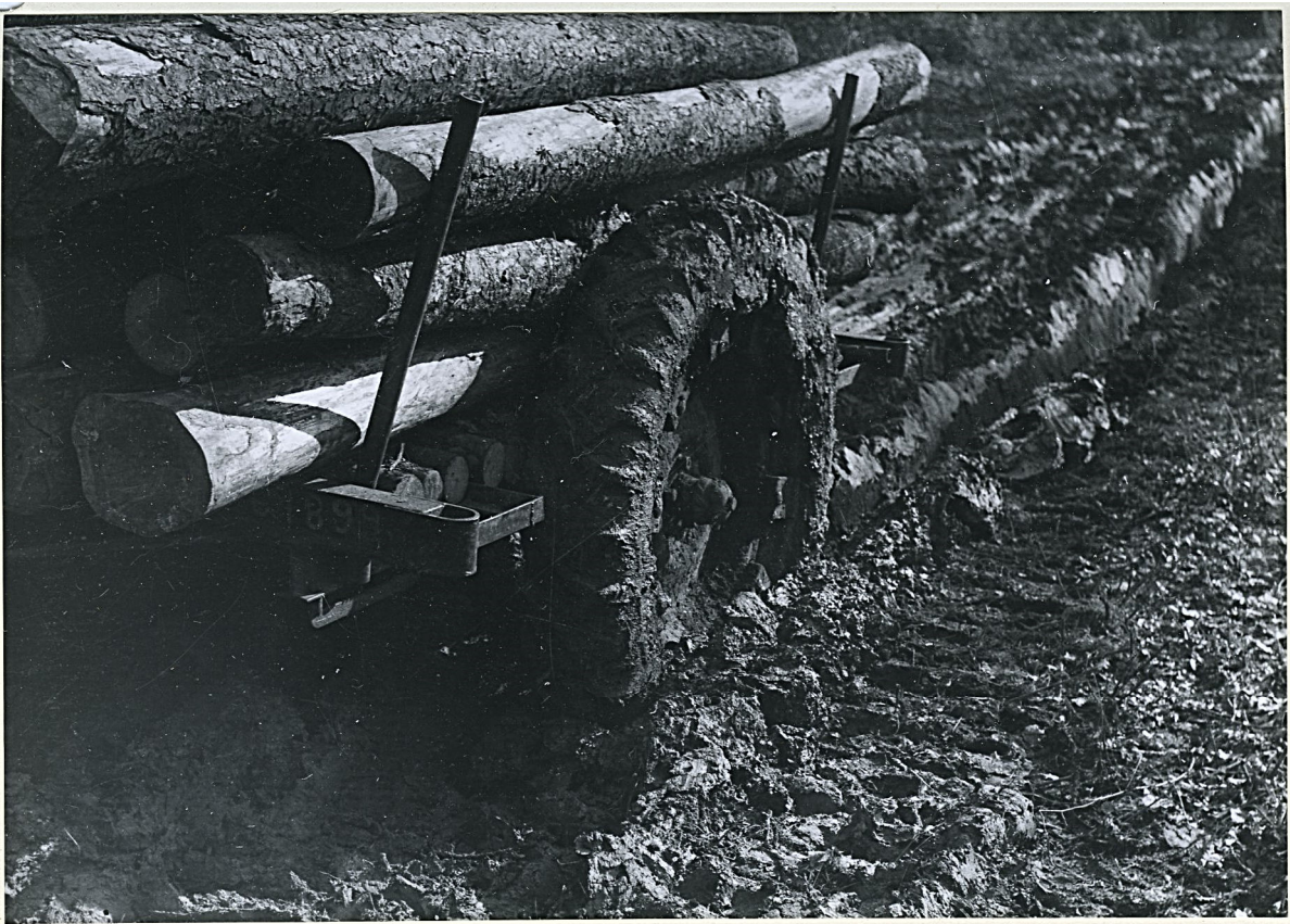
5. The two wheel trailer on 9 x 36 wheels rolling easily through soft wet clay. (Trial (a) Alice Holt).
