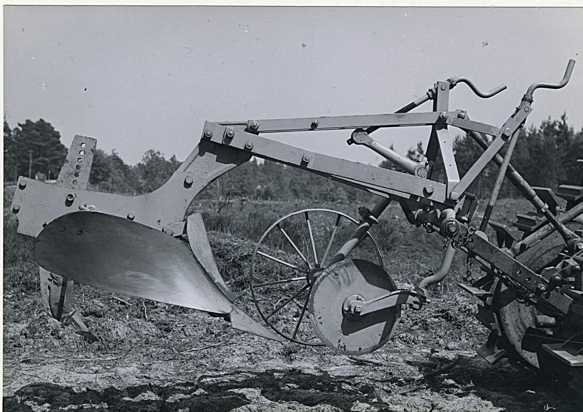
SIDE VIEW OF THE PLOUGH IN THE RAISED POSITION.
