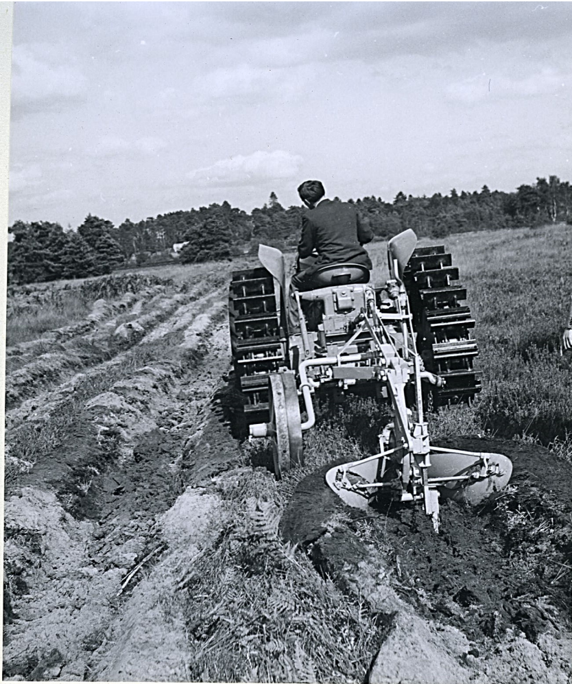
REAR VIEW SHOWING THE SLICES TURNED OVER ON EACH SIDE OF THE FURROW AND THE SUBSOILED PATH DOWN THE CENTRE.
