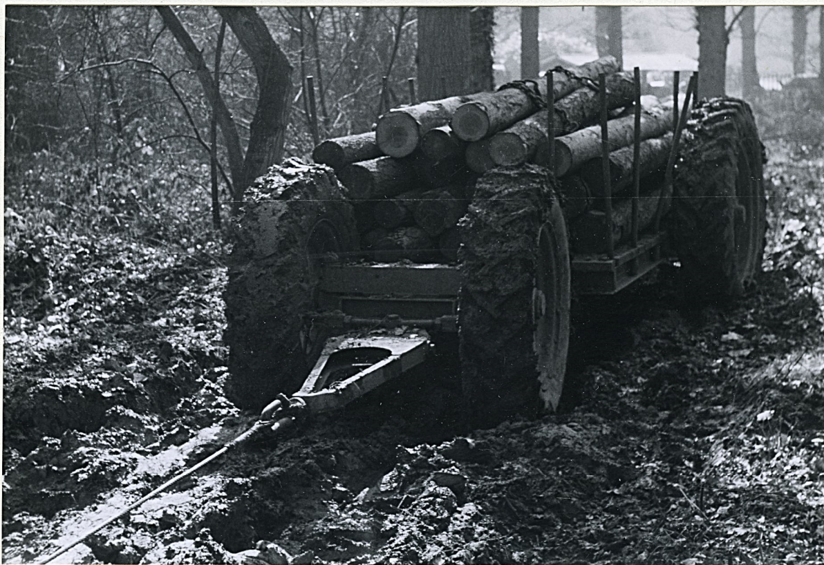
The trailer carrying a load of 2 tons during the rolling resistance tests.
