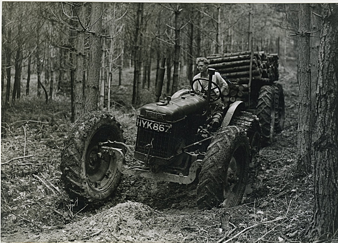
1. The first experiment based on one of the earlier model Fordson Majors here seen crossing a drain in a forest track. Front wheels are 11 X 36.
