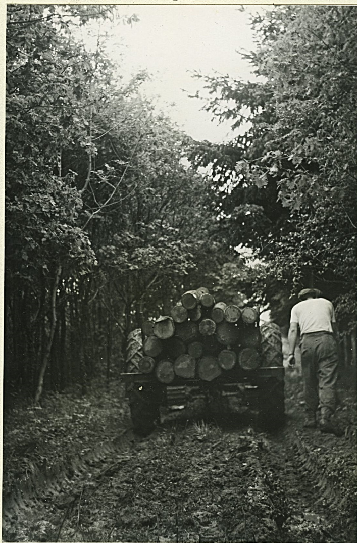
THE TRAILER WITH LARGE DIAMETER WHEELS EASILY PASSING OVER A SOFT WET RIDE.
