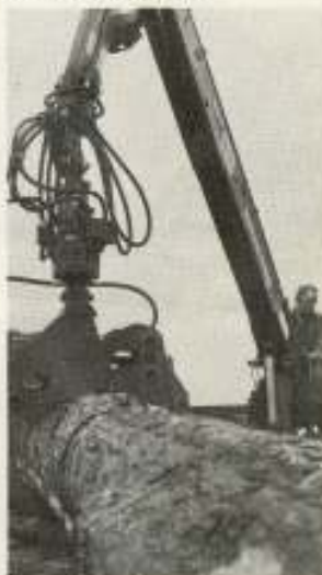
Note the single-lever control operating both clutch and winch-brake.
