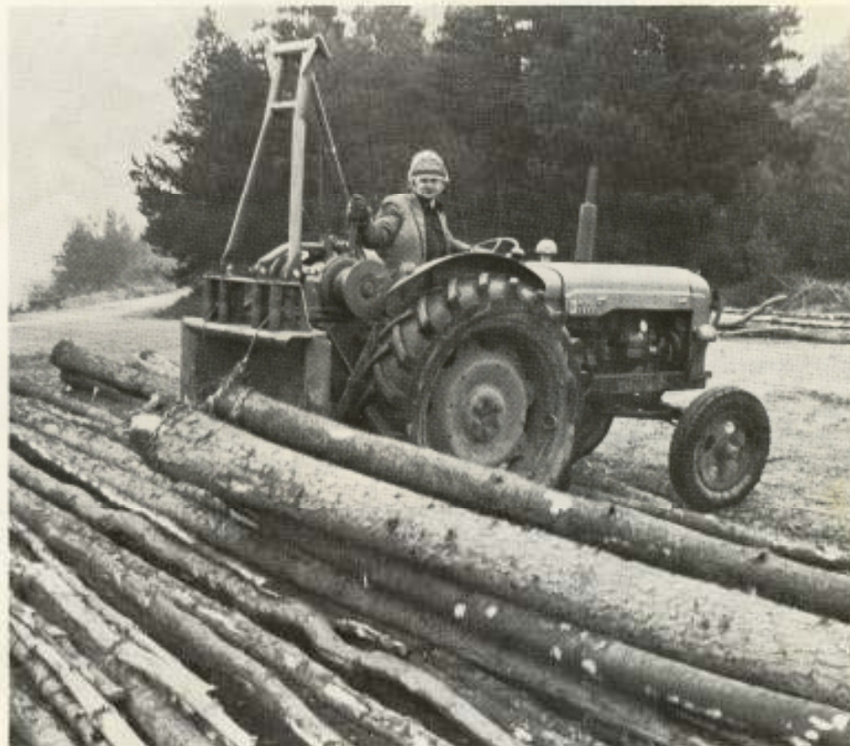
Jim Coulson with new double drum Igland Jones winch and highlead facility can keep a three man team of fallers fully occupied.
