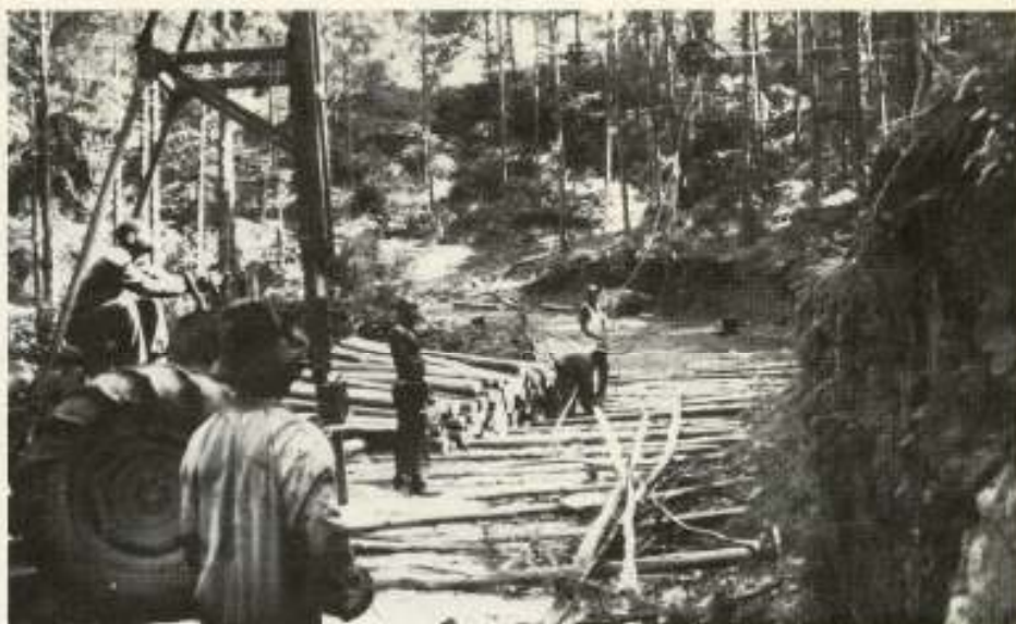
Igland Jones 4000/2 Skyline winching tree length eucalypt downhill and turning logs onto the road for cross cutting into pit prop length.
