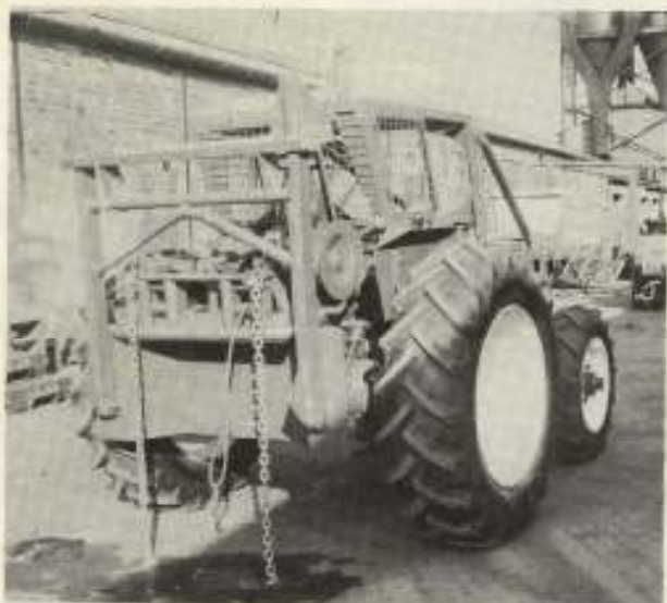
Highland County 4000/4 with double drum winch and ground anchors.
