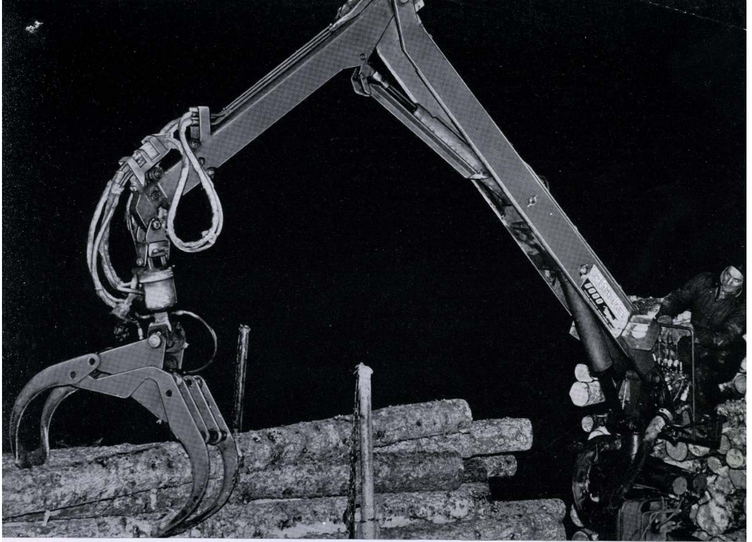
Rear mounting of the H.B. 5000 crane allows one vehicle to load another.
